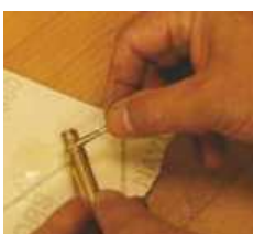
Spread the adhesive onto the tubes and twist them into the blanks
